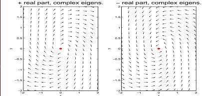
The bottom line: negative real eigenvalues or negative real parts means stability.
